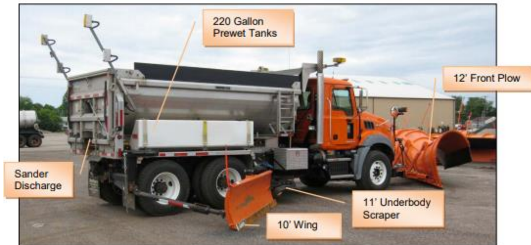
Figure 4.1 Winter road maintenance truck (Picture from Snow Plow Truck, NDDOT)
